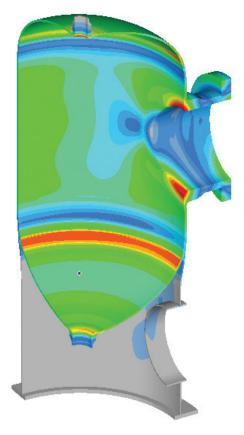
"Today, pressure equipment regulations allow us to apply a more accurate analysis method, using a tool like Simcenter Femap with Nastran for nonlinear calculations."
